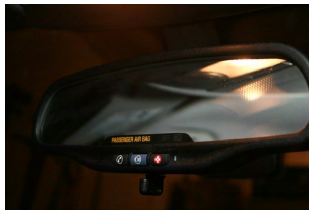
Figure 4-23 OnStar's three button interface provides access to hands-free calling, operator-assisted navigation and emergency services 98
