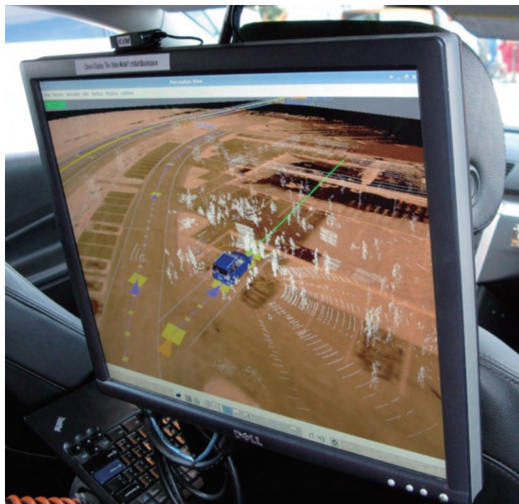
Figure 4-29 Sensors generate a three-dimensional map to aid navigation 117
