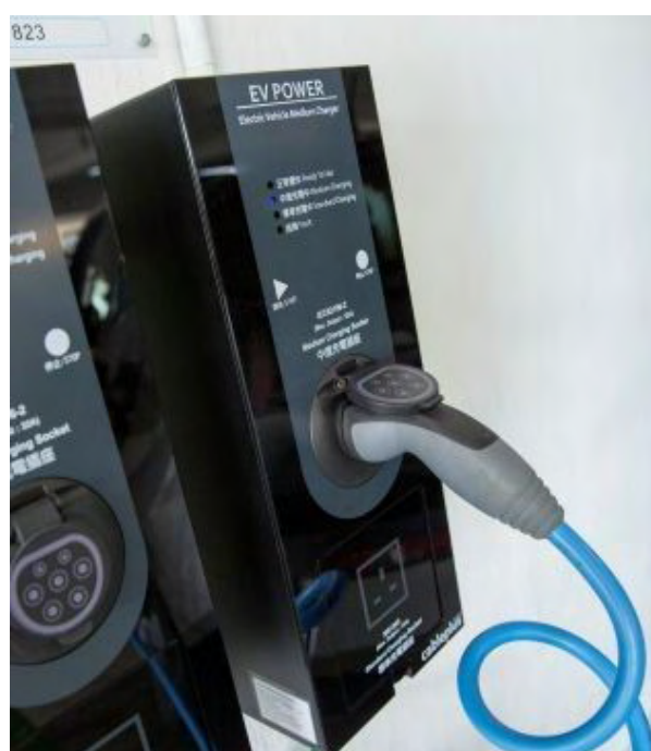
Figure 4-10 APAS& HKPC developed a semi-quick EV charging station called “Charging Pro” 74
