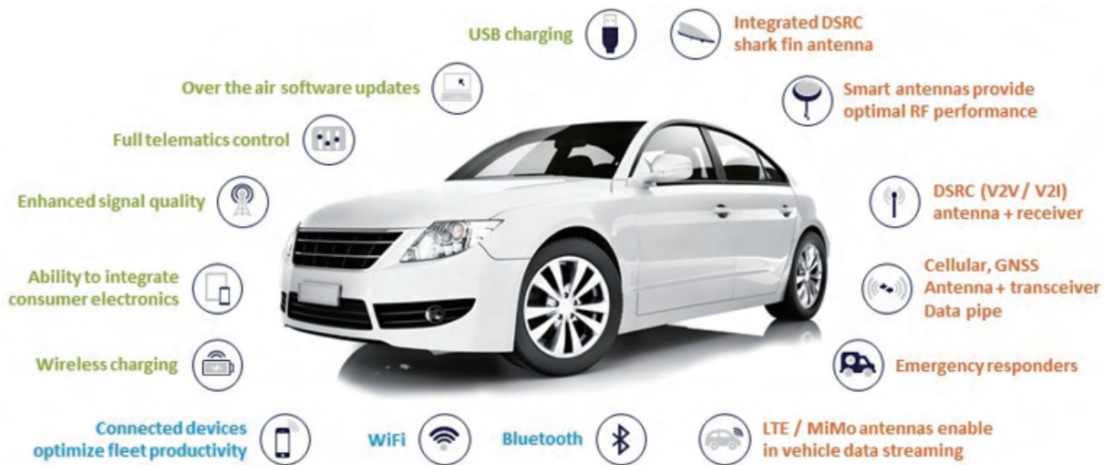
Figure 4-21 A connected car is equipped with several wireless transceivers like Wi-Fi, Bluetooth and LTE transceivers. 95
