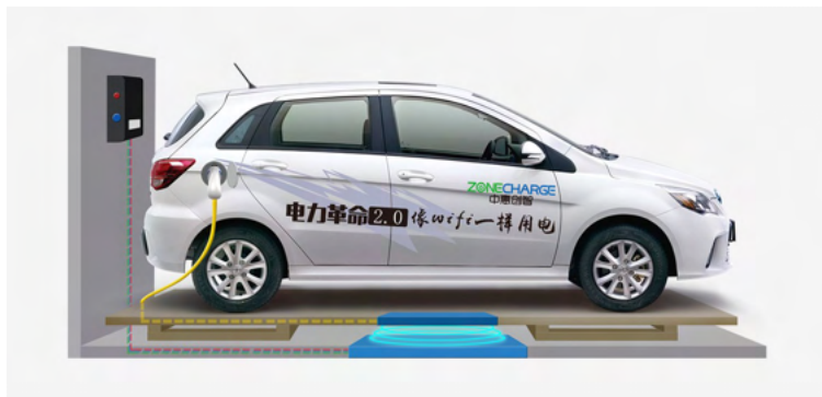
Figure 4-8 Zonecharge wired and wireless electric vehicle charging system 67
