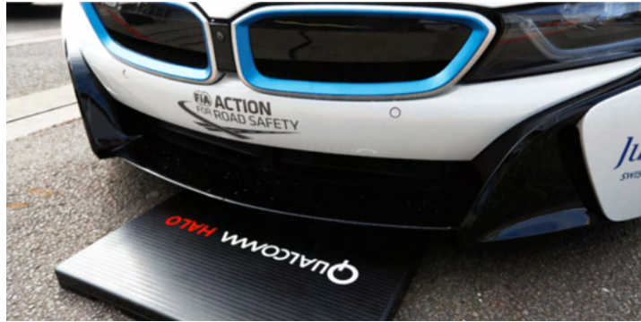
Figure 4-7 The Qualcomm Halo™ Wireless Electric Vehicle Charging System 65
